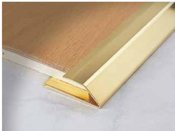
The WOODTEC LP profiles are specifically designed for finishing the perimeter of floating wood floors. The pointed, sloping shape of this profile ideally transitions to existing flooring or floors at lower elevations. The internal gap acts allows for differential movement. Installed with flathead screws.
